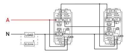
LED Indicator ON when Load OFF Active and Load at first Switch
